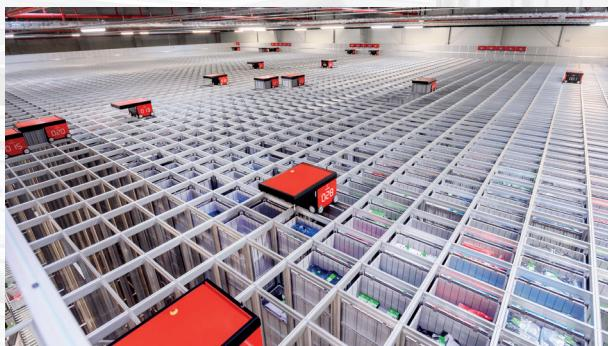
The heart of the logistics centre: The AutoStore system with over 50 robots. These control a total of 150,000 boxes with over 3.5 million products.
